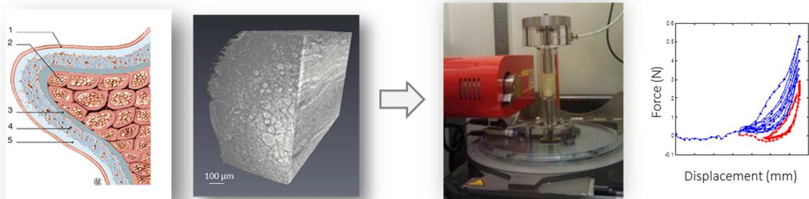
*Figure 1: (left) Scheme of a 2D frontal view of the vocal-fold tissue and 3D imaging using ESRF imaging; (right) Illustration of the mechanical device used for combined 3D in situ X-ray imaging.*
